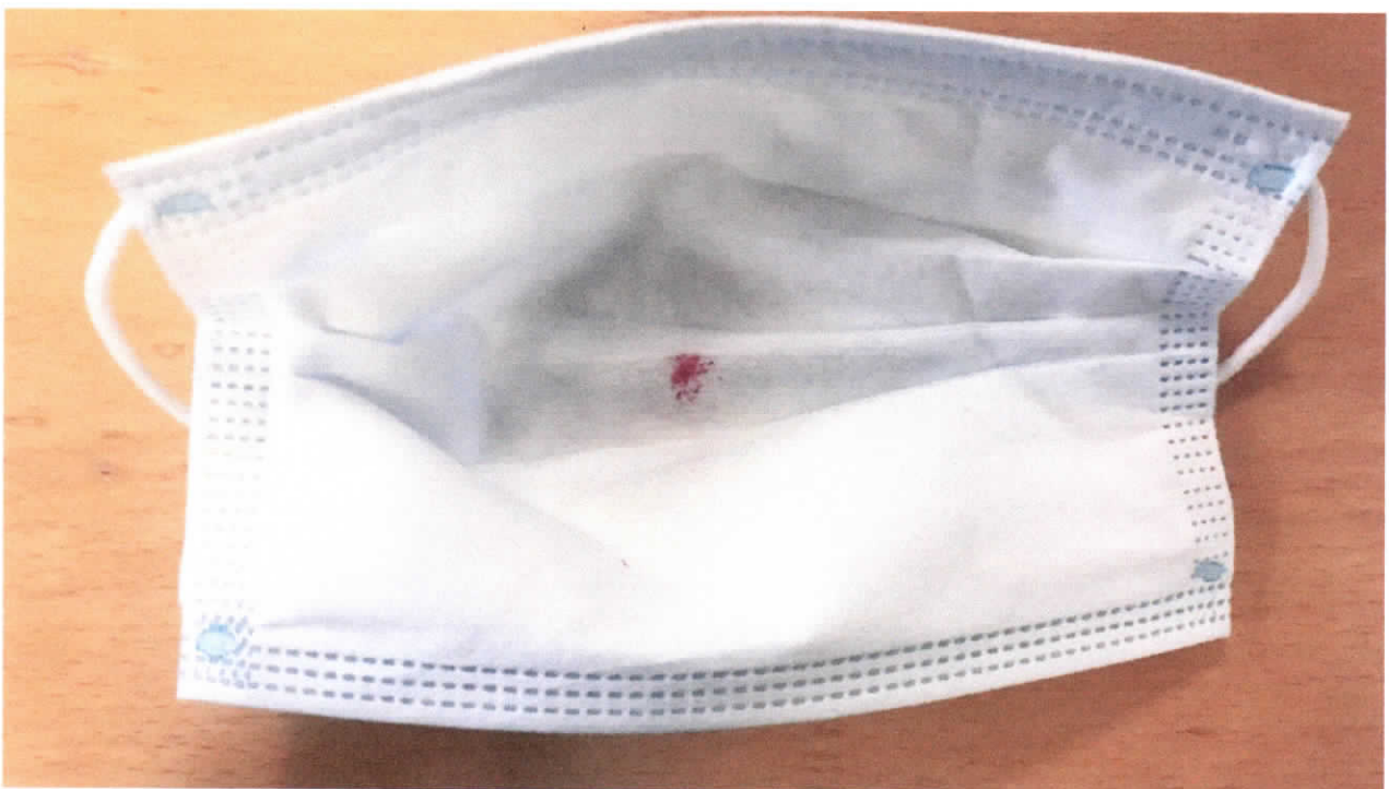
Figure 4 Back side of a mask after the test. The penetration is clearly visible as a red spot
